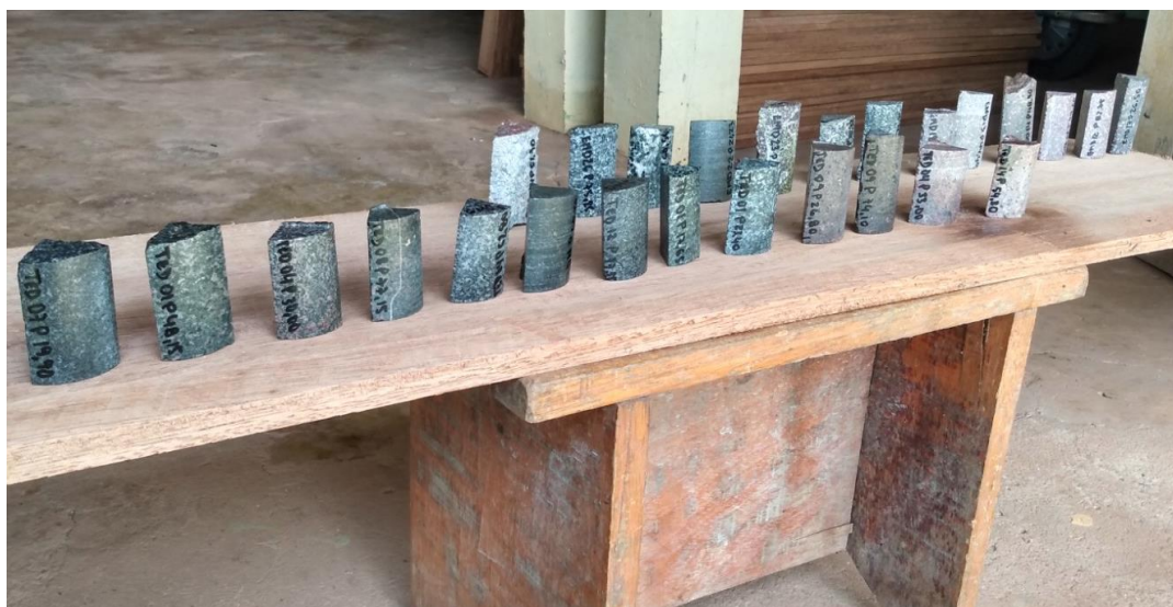
Figure 3: drill cores used in petrographic analysis
