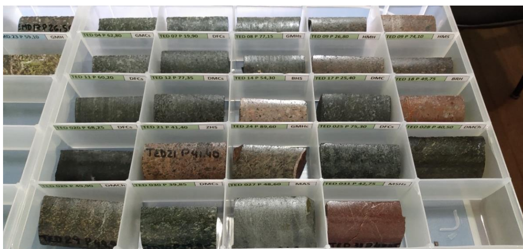
Figure 2: drill cores used in petrographic analysis
