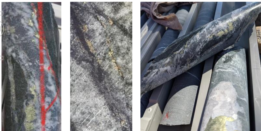
Figure 4. Osprey IOCG copper mineralisation (chalcopyrite) in drill core.
