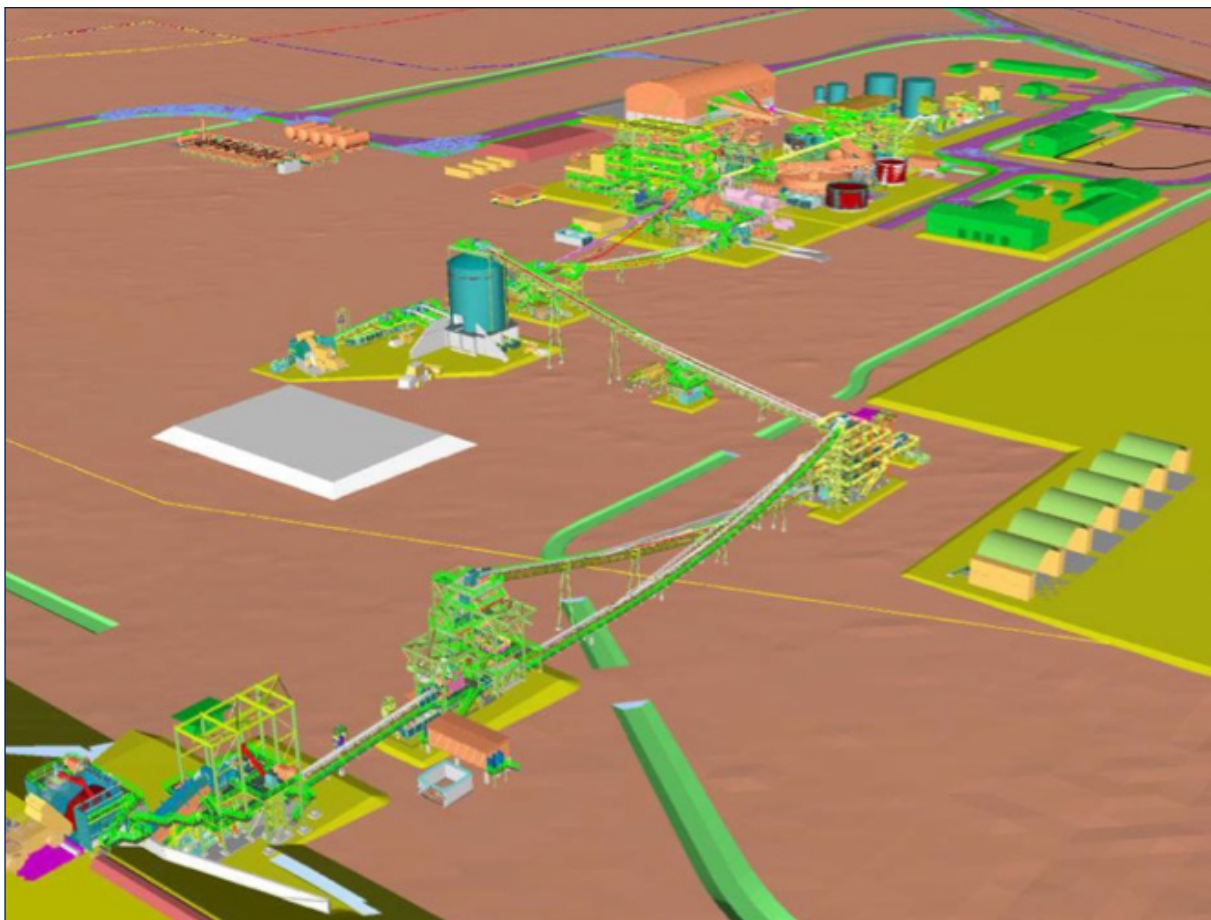
Figure 4: Revised Process Plant layout incorporating closed circuit crushing and large fine ore bin
