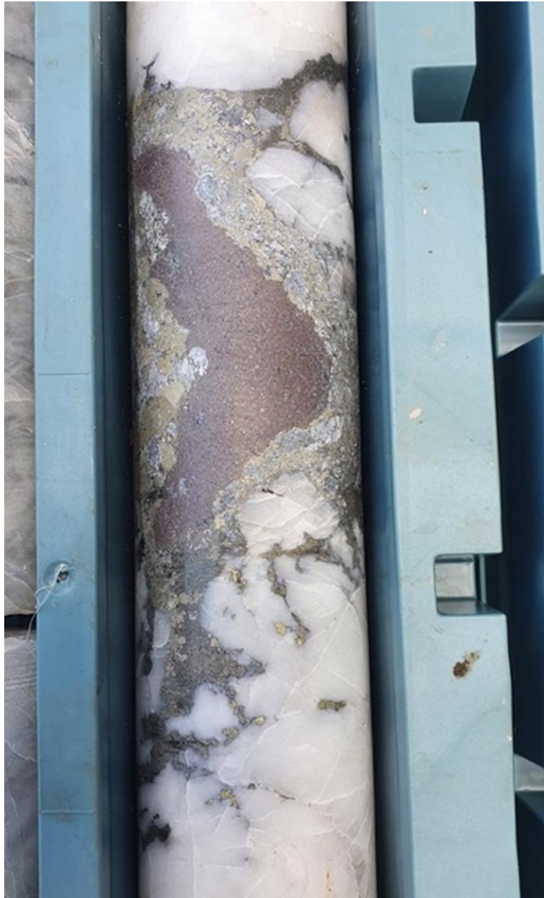
Figure 10. Hole 2: Zinc rich (pink sulphide) and copper rich (yellow sulphide) massive sulphide mineralisation at 168.13m which forms part of the 19m downhole intersection.
