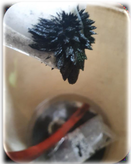
Figure 9: Magnetic Concentrate - Magnetic particles attracted to a hand magnet from the upper saprolite.
