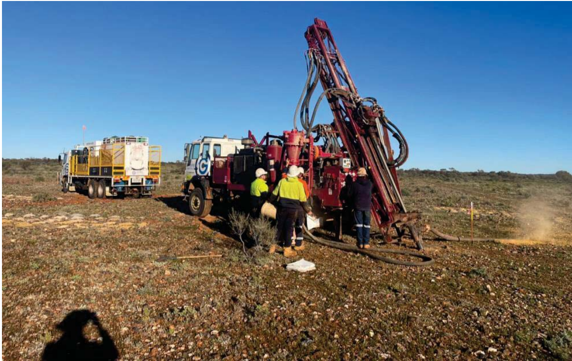
Figure 8: Aircore Drilling Rig at Everlong Prospect of the Austin Gold Project
