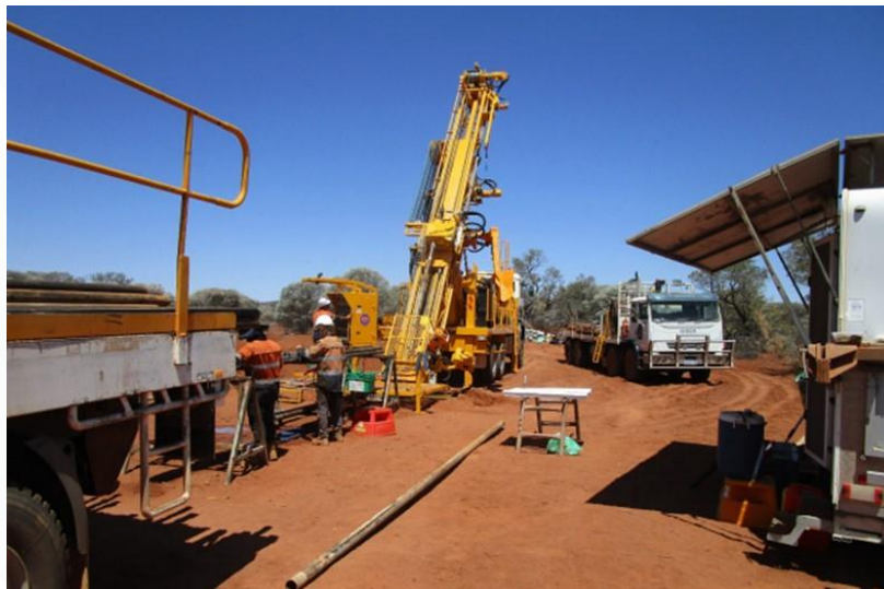
Figure 8 – Stage 8 core rig drilling
