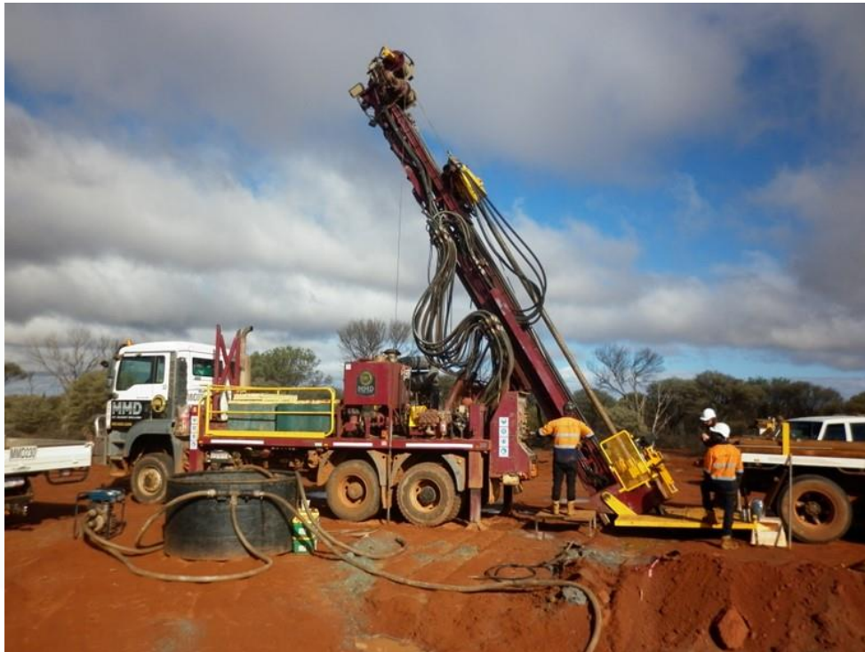
Figure 12 – Stage 10 diamond core rig drilling core tails
