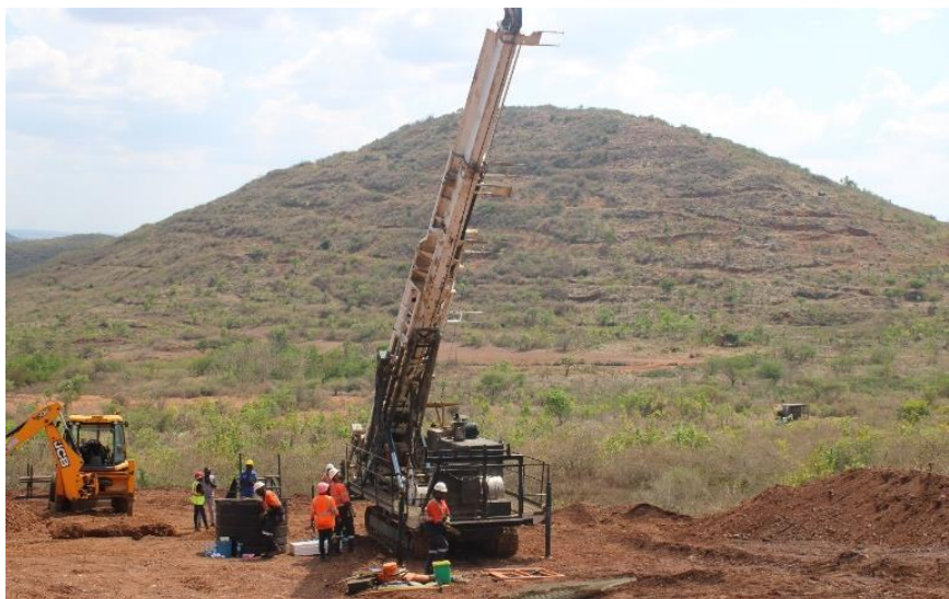
Diamond Drill Rig with Nyanzaga Hill in Background
