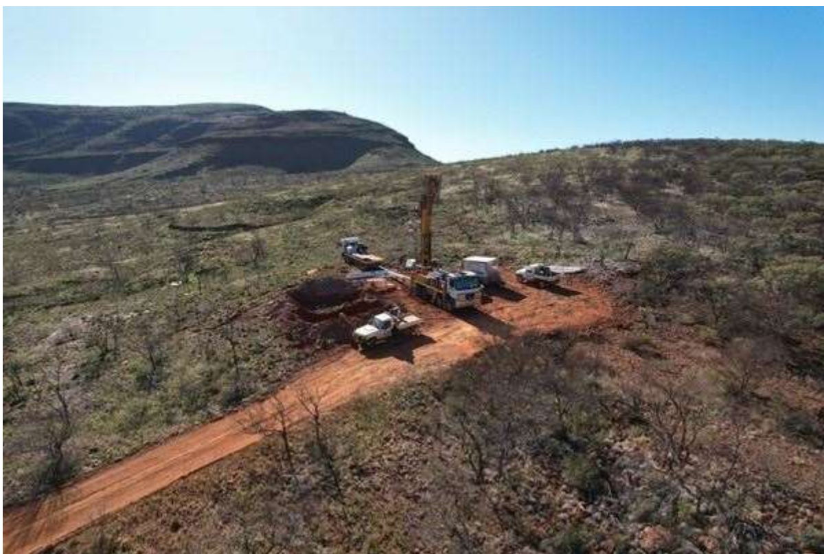
Figure 2 - Diamond drill rig drilling at the Hellcat Teano prospect
