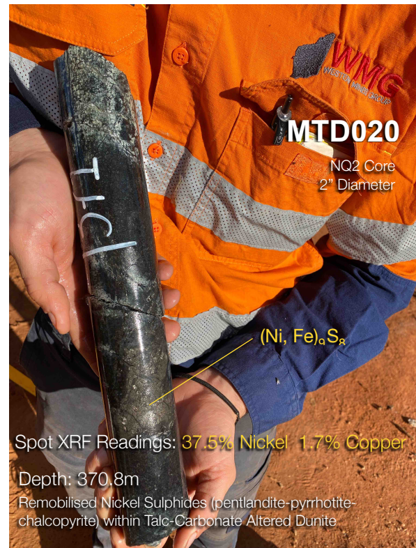
Figure 3: Photos showing examples of visible sulphides from Mulga Tank drilling program Note: core is NQ2 being 2 inches or 50mm diameter
