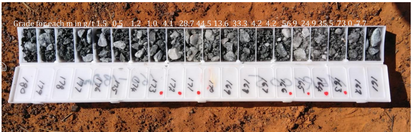
Figure 4: Chip tray from MERC005 with 16m @ 20.92g/t high grade intercept from 161m
