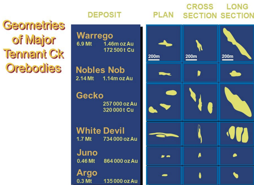
Figure 5: Geometries of Major Tennant Creek Orebodies, noting the typical constrained plan/horizontal footprint.
