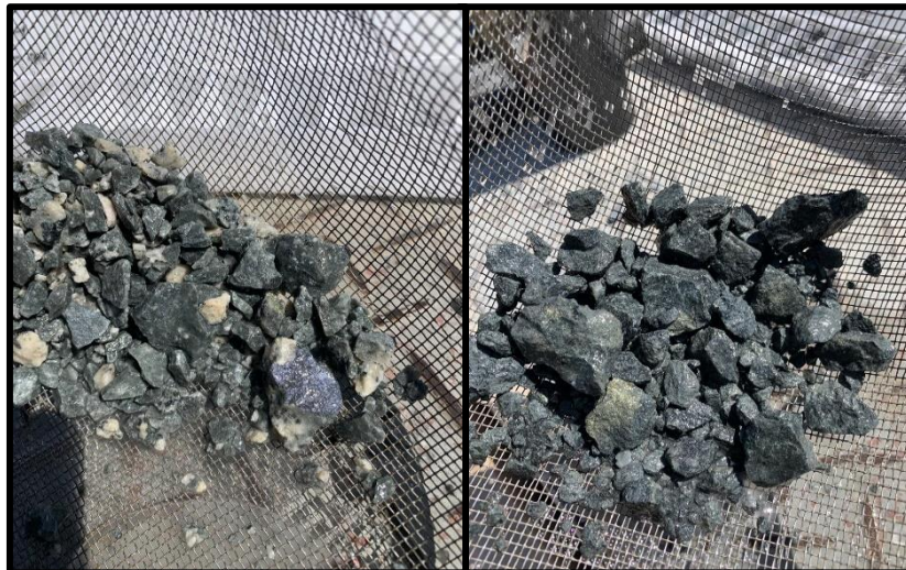
Figure 3. Bommie Prospect: Drill chips showing albite, chlorite, biotite, disseminated sulphides and quartz-carbonate veins.
