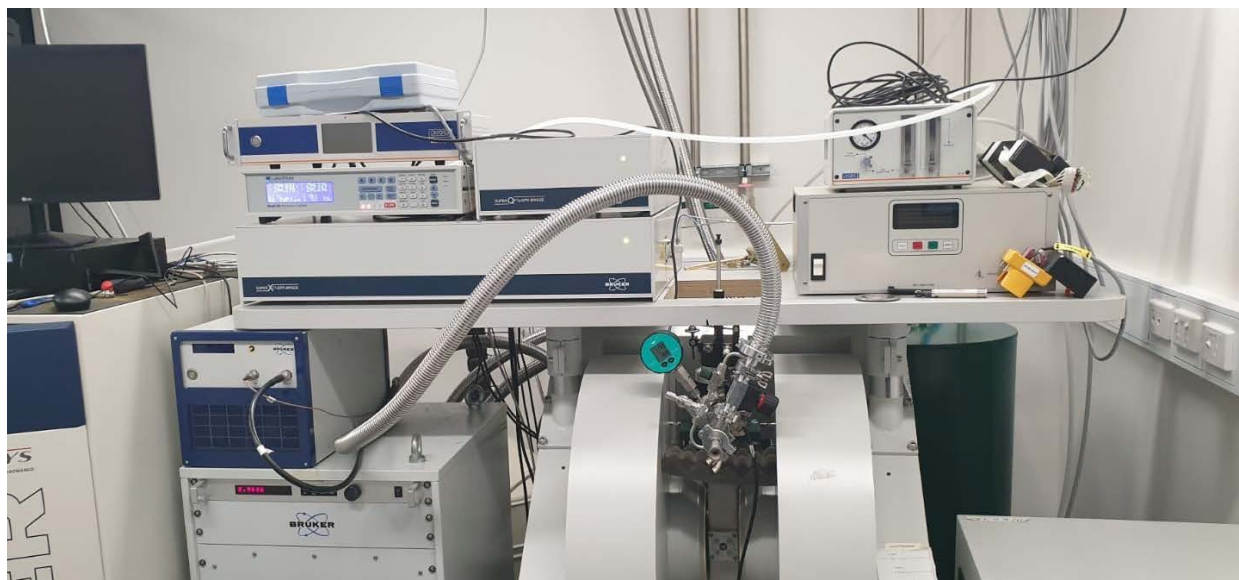
Electron spin resonance setup to validate qubit robustness.
