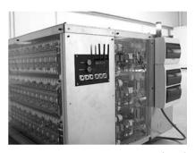
Battery Energy Storage System (BESS) made with EV cells
