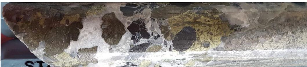
Figure 8: Chalcopyrite-pyrite-sphalerite mineralisation hosted in a quartz-carbonate vein in strongly sericite-altered granodiorite in drill hole BRUDD001 (13.9 – 14.1m)
