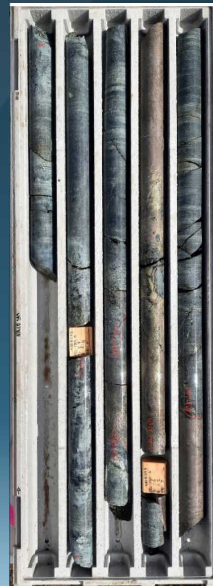
Massive sulphide mineralisation at 190.6m downhole in NRCD293
