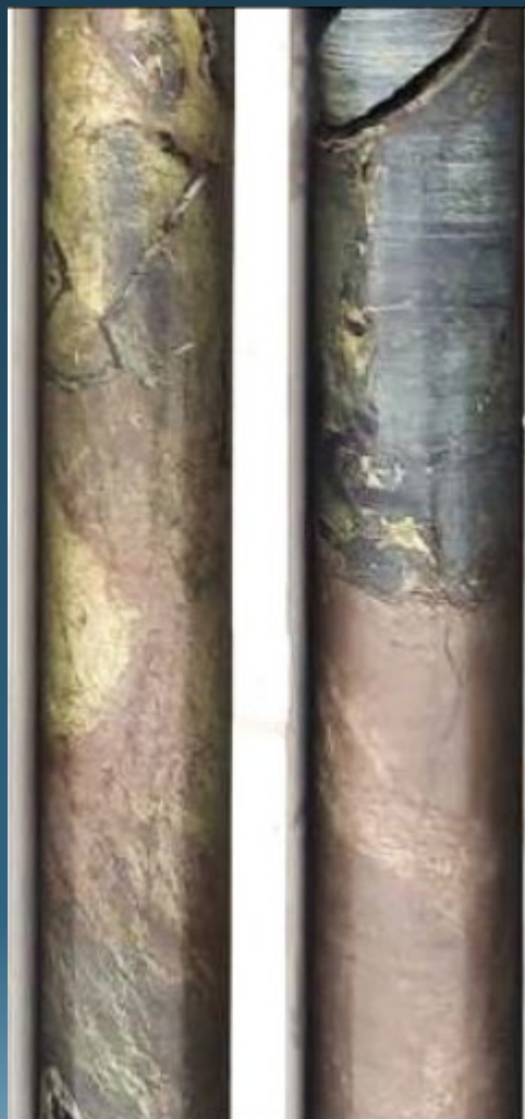
Massive sulphide mineralisation at 190.8m downhole in NRCD293
