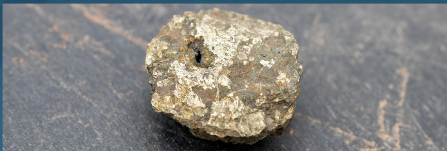
Massive sulphide intercepted in aircore drilling at Jimberlana
