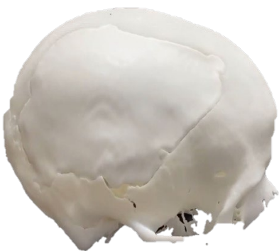
3D Printed Cranial Implant designed by SHG AI Model
