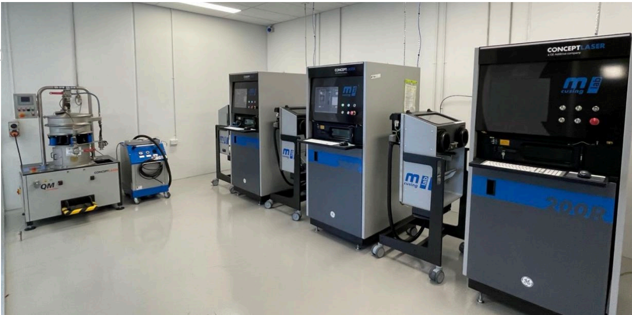
Three Titanium 3D printers installed at AE Medical Manufacturing facility in Melbourne
