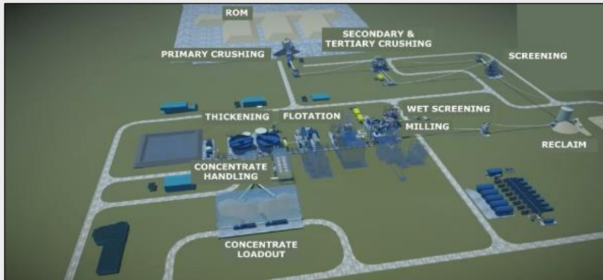
Goulamina Process Plant Layout
