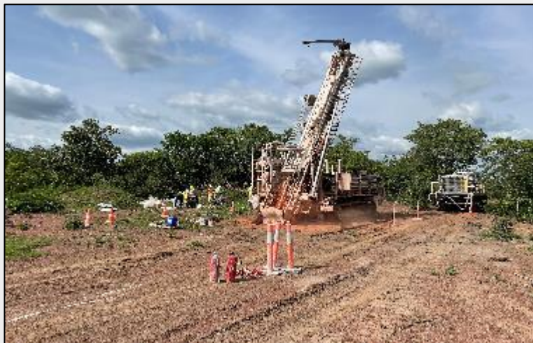
RC rig drilling pre collars
