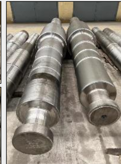
Rough machining of ball mill pinion shaft finalised in China
