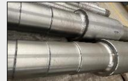
Rough machining of ball mill pinion shaft finalised in China
