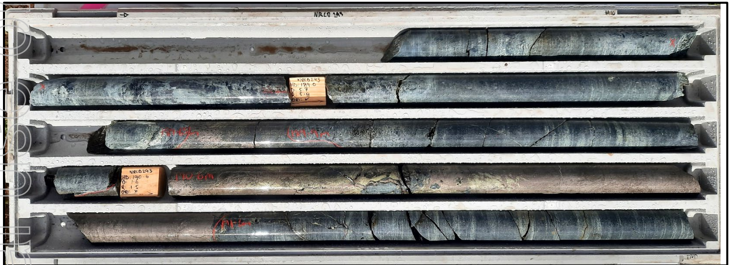
Figure 7 — NRCD279 drill core tray with disseminated sulphide mineralisation from 265.9m to 269m, part of a broader disseminated mineralised zone between 234.9m and 269m. See Appendices 1,2 & 3 for drill hole details including preliminary visual logging of sulphide mineralisation.
