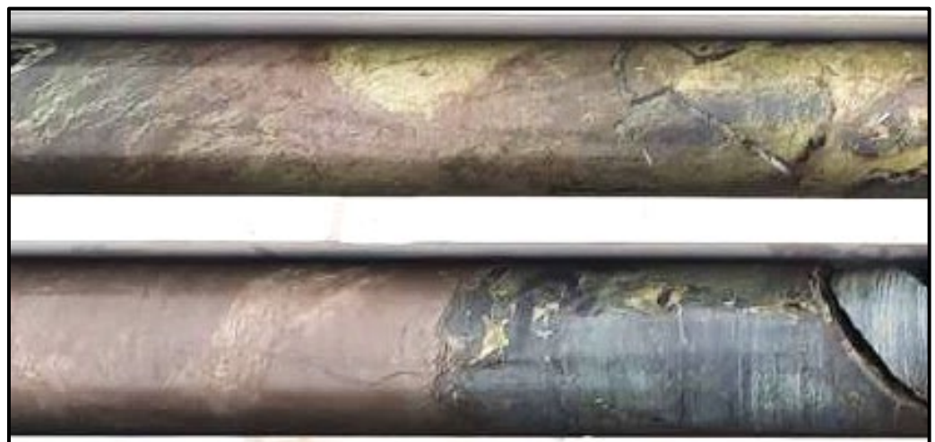
Figure 1 – Detail of massive sulphide mineralisation at 190.8m downhole in NRCD293 (field of view approximately 25cm across, NQ2 core) 1
