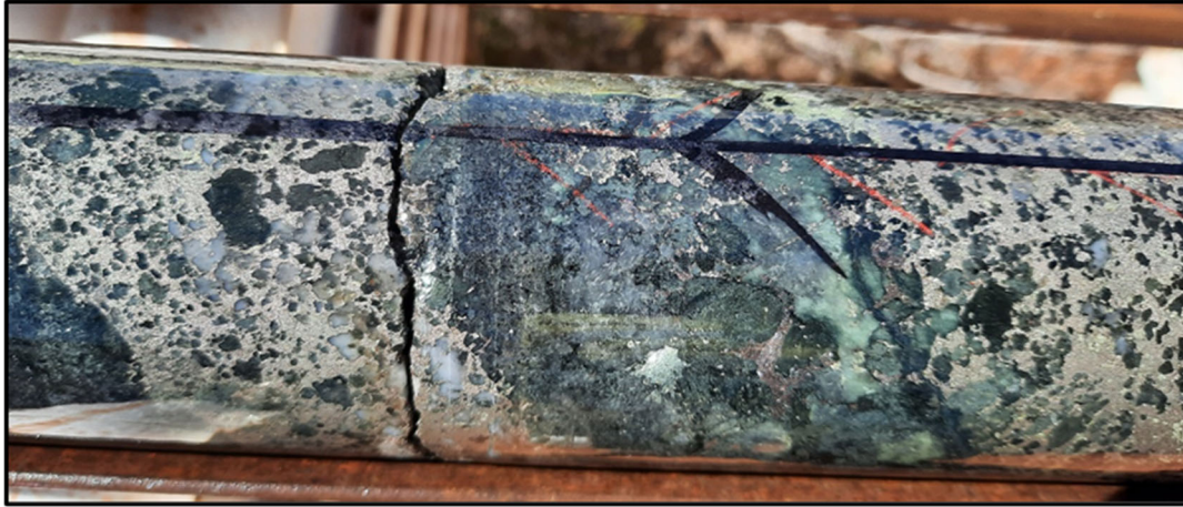
Figure 14 - Matrix sulphide mineralisation at 399m downhole in DBDD001 (field of view approximately 20cm across)
