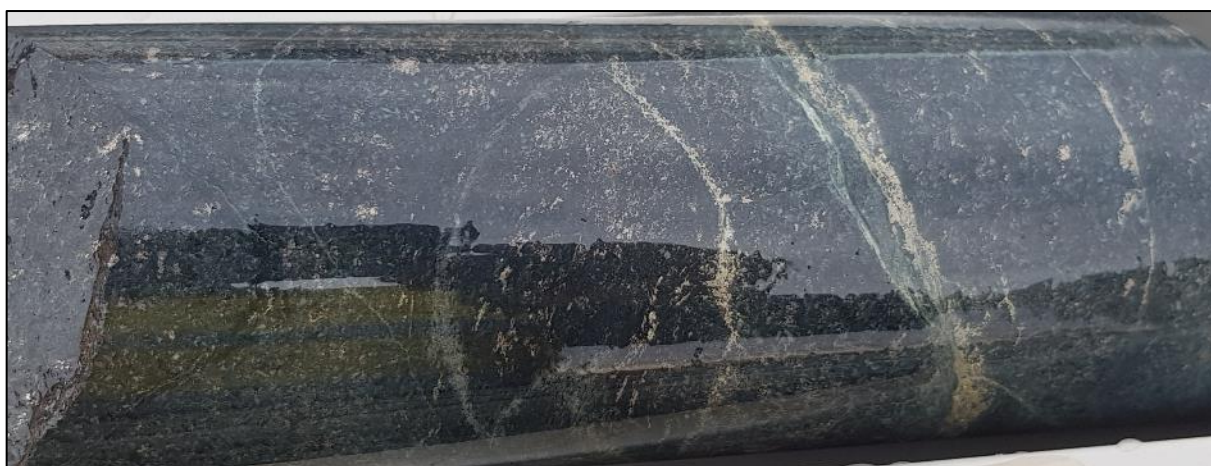
Figure 19: FMDD0042 ~588m Typical of the disseminated and stringer pyrite and pyrrhotite observed in all three holes at Recon 1, occasionally chalcopyrite is also observed within these disseminated zones.
