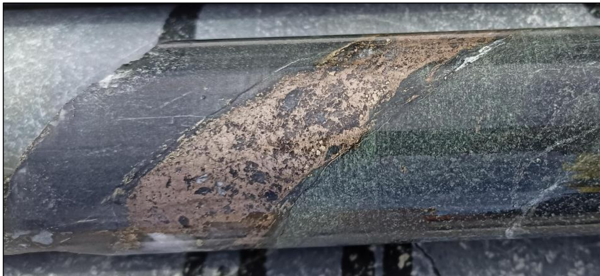
Figure 17: Pyrrhotite vein in altered andesite within hole FMDD0030.
