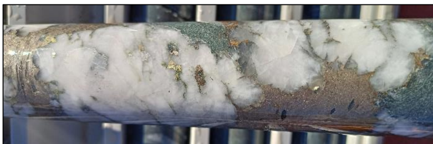
Figure 1: FMDD0047 ~231m, sulphide bearing quartz vein with pyrrhotite, pyrite, arsenopyrite and chalcopyrite hosted within andesite volcanics.
