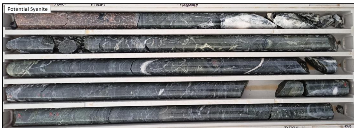
Figure 16: FMDD0047 ~128m Possible syenite intrusion surrounded by zones of sulphide bearing alteration, increased structural disruption and elevated vein density.
