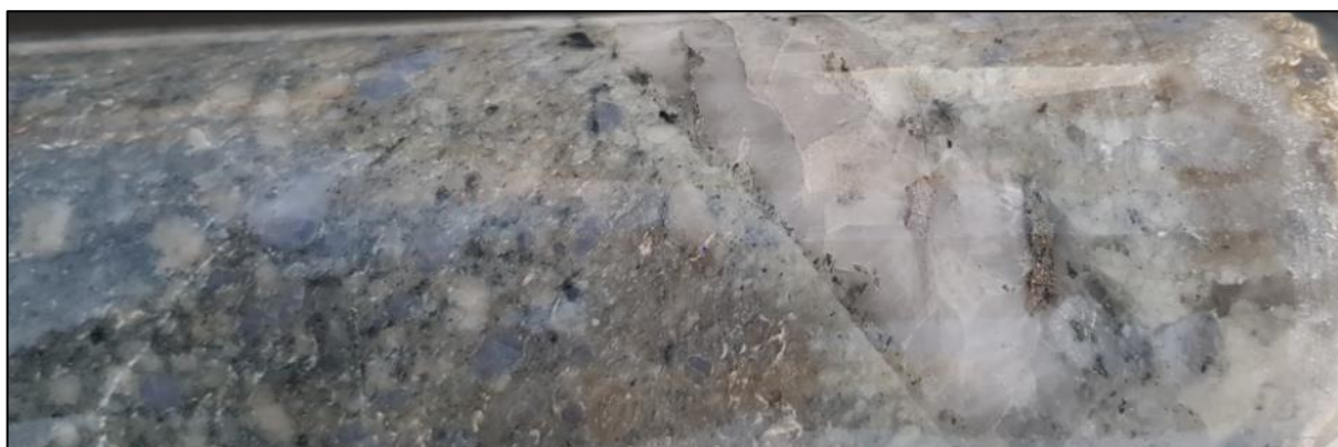
Figure 18: FMDD0042 ~66m Arsenopyrite and pyrite bearing quartz vein within altered felsic porphyry.
