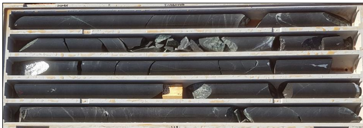
Figure 14: FMDD0047 ~510m for comparison an unaltered andesite with minimal veining and without felsic to intermediate intrusions. Alteration, veining and mineralisation at Recon 1 appear to have an association with the porphyry intrusions.
