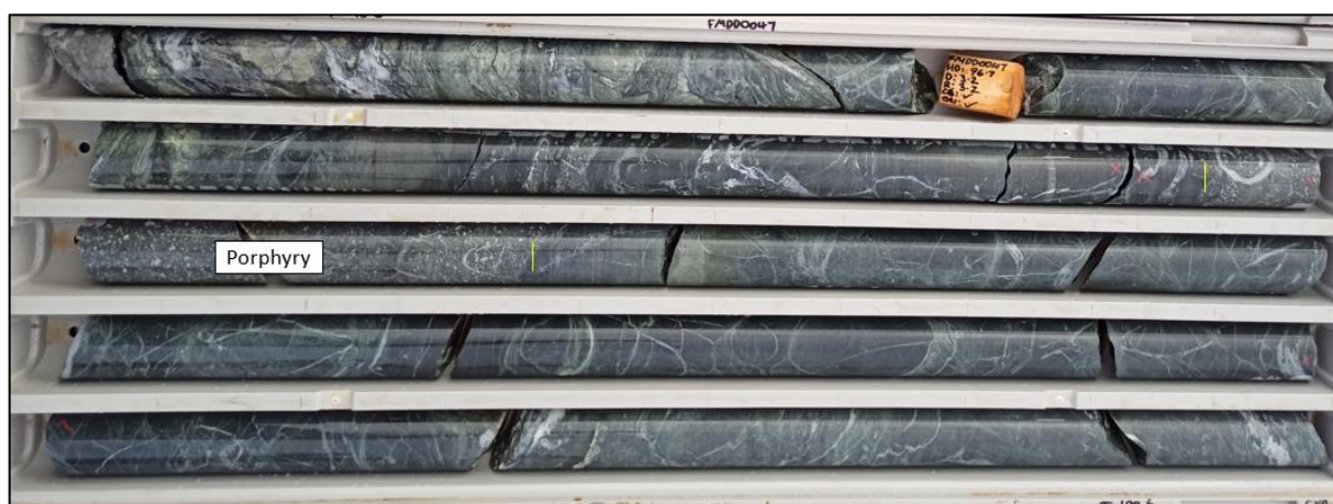
Figure 15: FMDD0047 ~98m Altered porphyry surrounded by zones of sulphide bearing alteration, increased structural disruption and elevated vein density.
