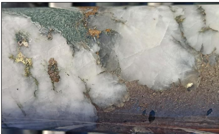
Figure 2: Close up view of the mineralised vein in Figure 1 . Veining with this sulphide assemblage is known to host gold in the Laverton-Leonora District.
