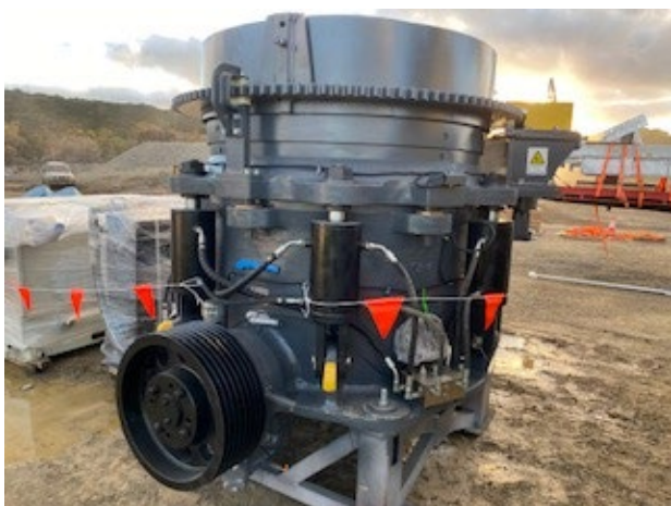
Figure 5 - Secondary Cone Crusher Delivered
