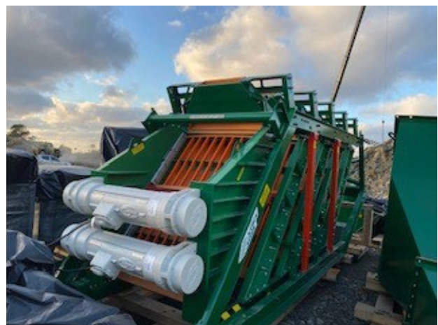
Figure 6 - Derrick Screen Delivered
