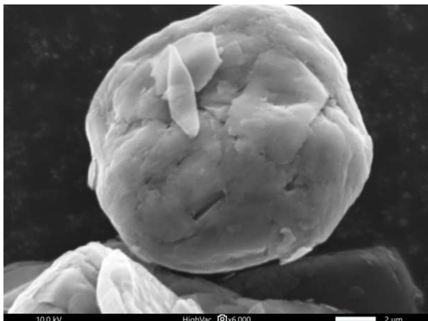
Figure 2: SEM analysis of Chilalo's thermally purified uncoated spherical graphite
