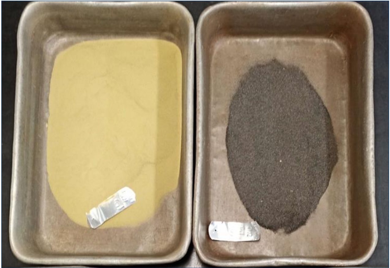
Figure 17: Rare earth (LHS) and heavy mineral concentrate (RHS) streams from wet shaking table tests after flotation.
