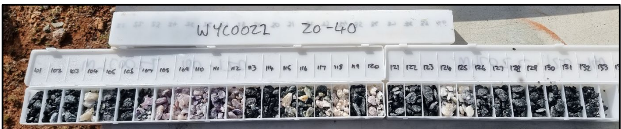
Figure 3: Hole WYC0022 (101 to 132m) note the pegmatite zone with metagabbro layers, between 107 and 125m depth characterised by lepidolite and possible eucryptite (hydrothermal alteration product of spodumene) mineralisation.
