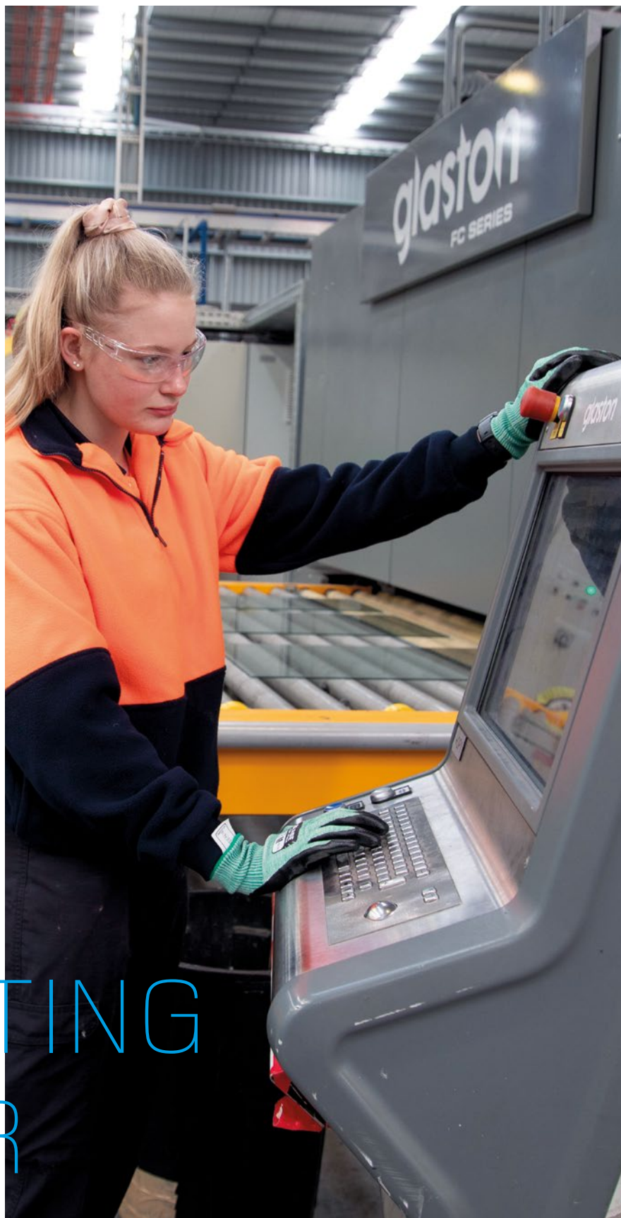
Furnace Operating, Producing Toughened Safety Glass
