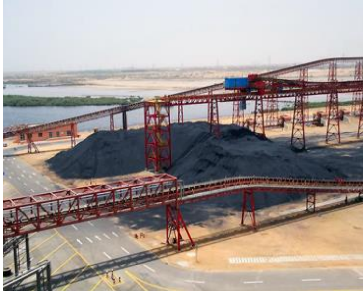
Figure 19: Typical mobile tripper stockpile elevated belt conveyors
