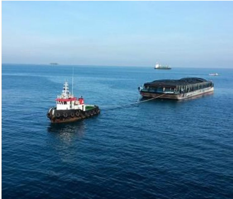
Figure 21: Tugboat towing an ore transshipment barge
