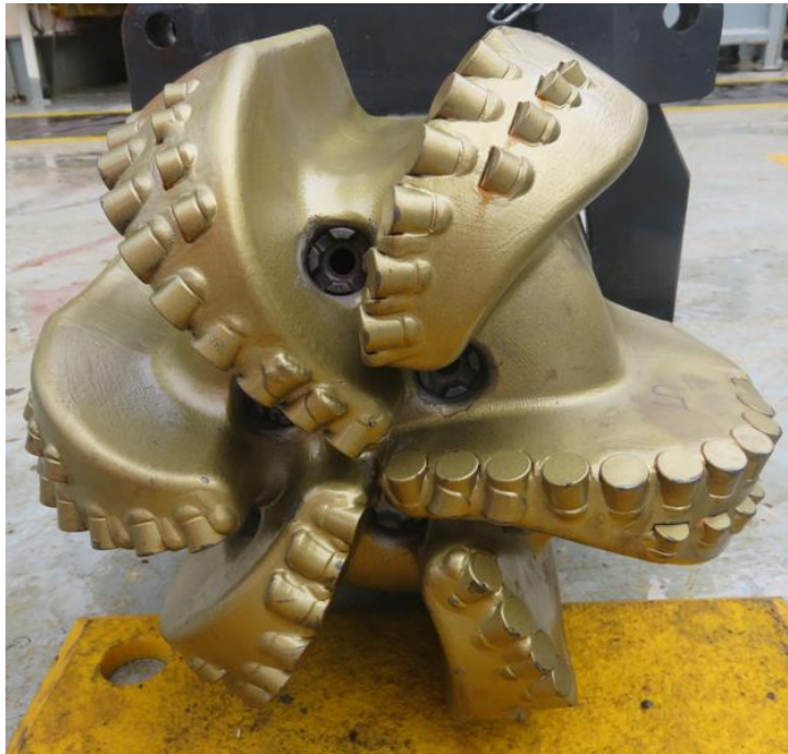
12-1/4" drill bit that will be used to drill the target reservoir section
