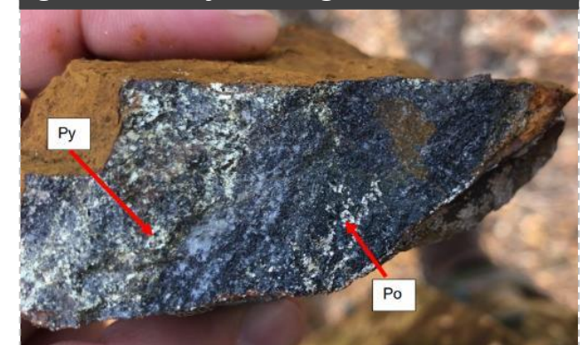
Mineralised pyrite (py)-pyrrhotite (po) gneisses at Tysklandgruve
