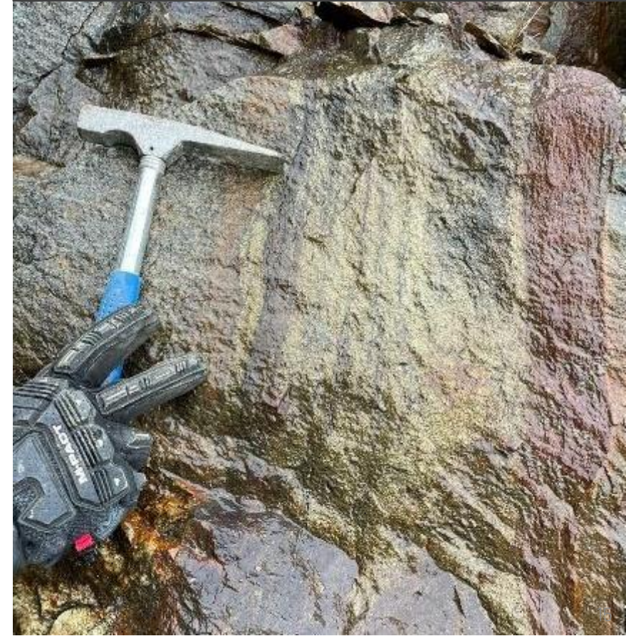
Massive, impregnated sulphides (pyrite, chalcopyrite, pyrrhotite) at the Route 3 road outcrop on the Northern Nyberget license (556297/ 6953183/ 382m)
