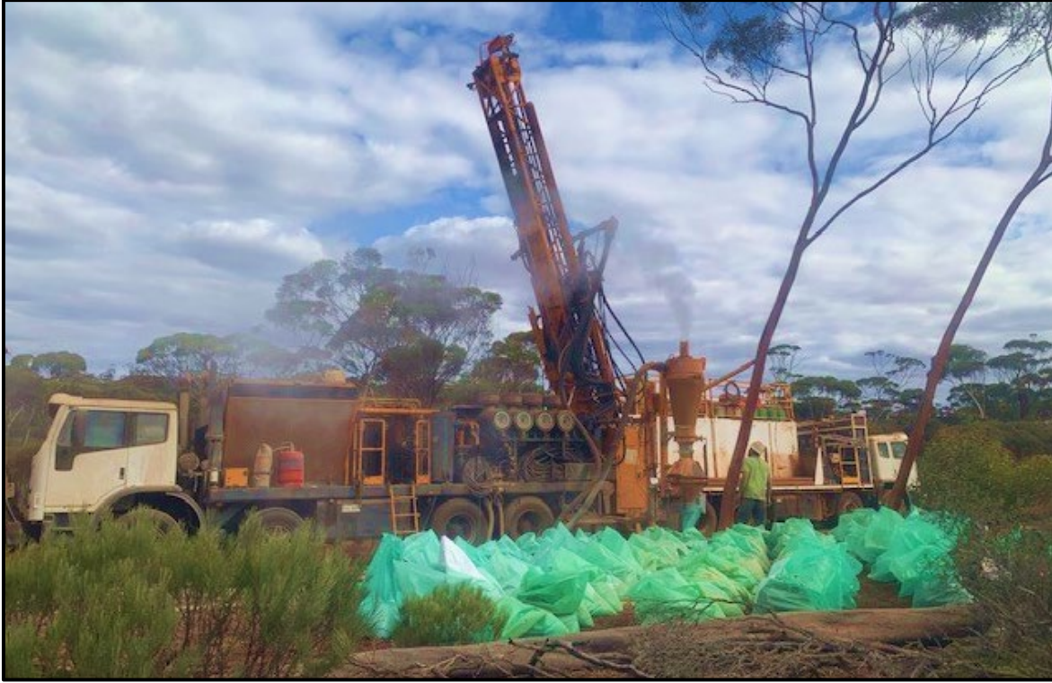
Figure 5 – RC Drilling at Callisto, Norseman 2022
