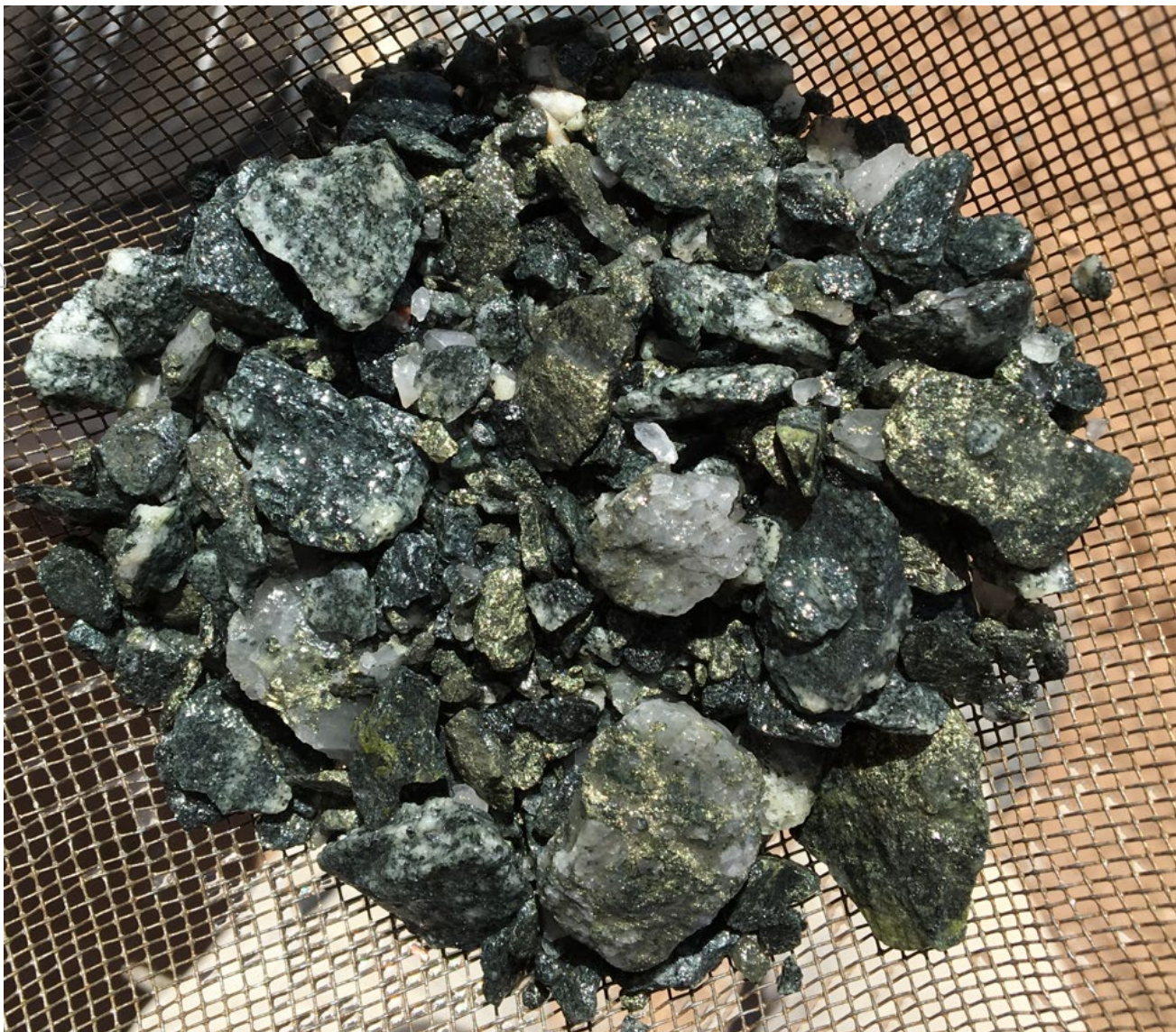
Figure 2: Chalcopyrite and pyrite mineralisation in hole 22CARC014 (234-235m) in RC percussion drill chips.
