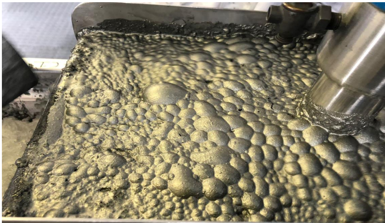
Figure 3: The sulphide flotation kinetics are extremely rapid indicative of a largely sulphide orebody
