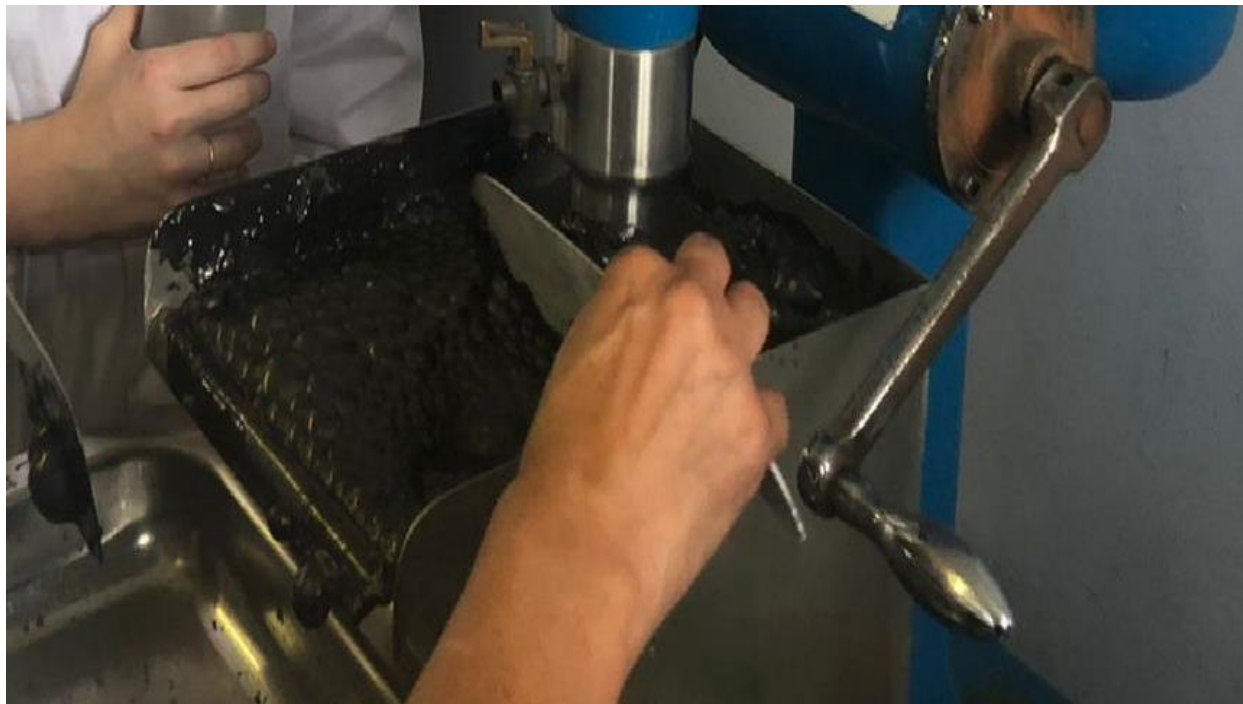
Figure 2: Carbon flotation indicates high flotation kinetics
