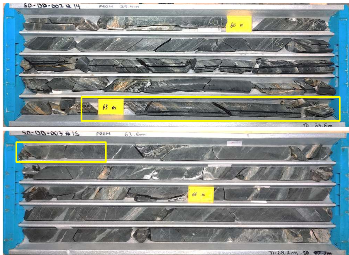
Figure 1 Drill-core from SODD003. The sample interval assaying 42.8g/t gold is highlighted in yellow.
