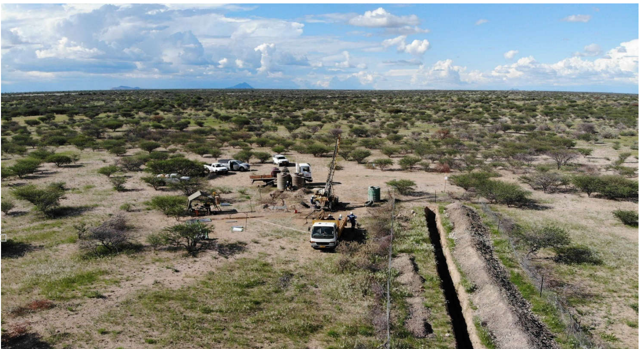
Figure 3 – Diamond drill rig alongside Trench 5
