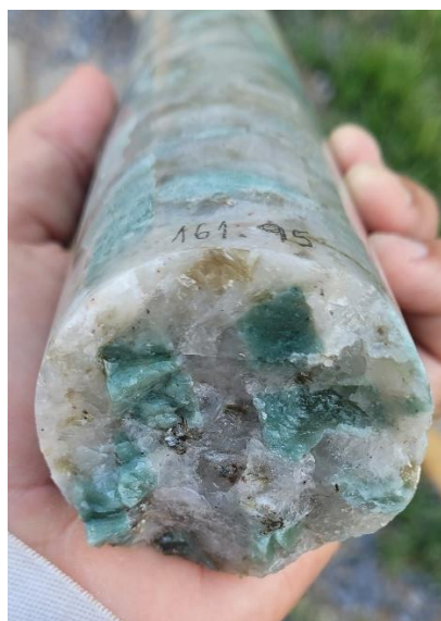
Figure 1: SADD005 – large, fresh green spodumene crystals in drill core
