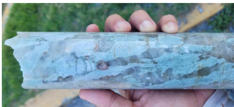
Figure 1: SADD005 – large, fresh green spodumene crystals in drill core
