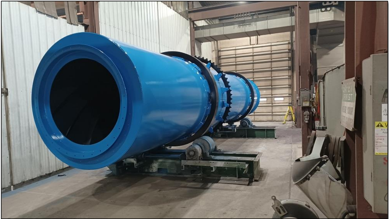
Figure 3 - Cabinda Phosphate Plant - Completed cooler drum ready for export.
