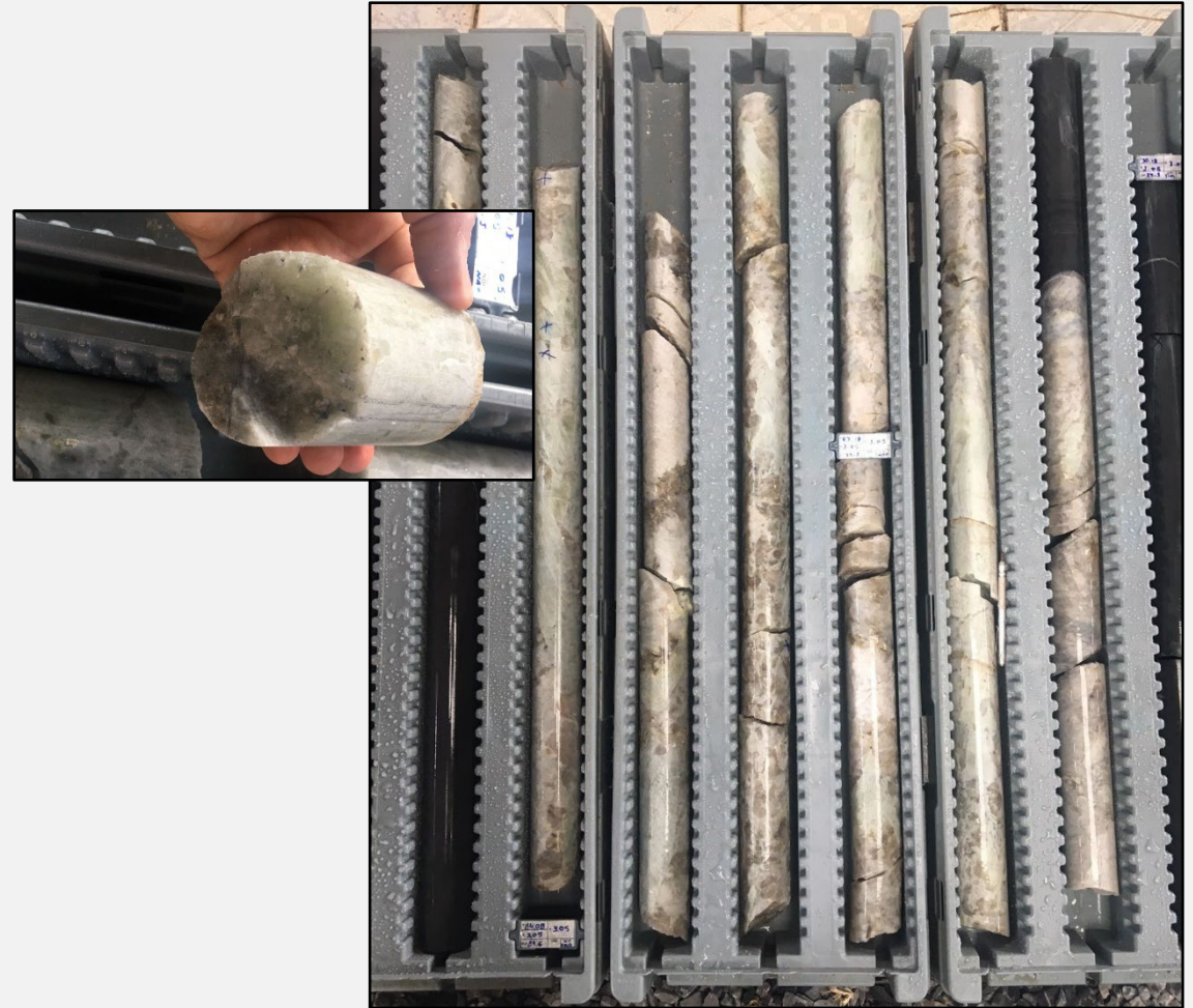
Figure 2: SADD001 - 5.25m thick coarse-grained pegmatite (83.85-89.10m), containing abundant light green spodumene crystals, hosted within a biotite-quartz schist (black rock)
