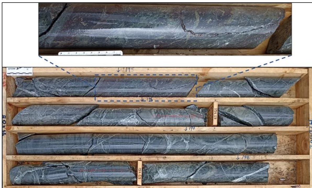
Plate 3. Copper Duke Project – Borehole HTD002 – Details of abundant sulphides (pyrrhotite, pyrite) and magnetite-quartz±chalcopyrite veining (~196 m depth).
