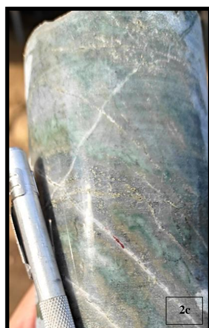
Plate 1: HTD001 core (31.64m to 35m interval), intersecting andesitic volcanic with partially oxidised quartz-pyrite stockworks and narrow quartz-pyrite-chalcopyrite veinlets
