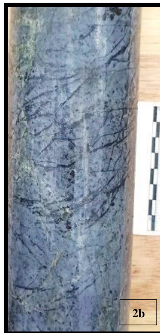
Plate 1: HTD001 core (31.64m to 35m interval), intersecting andesitic volcanic with partially oxidised quartz-pyrite stockworks and narrow quartz-pyrite-chalcopyrite veinlets
