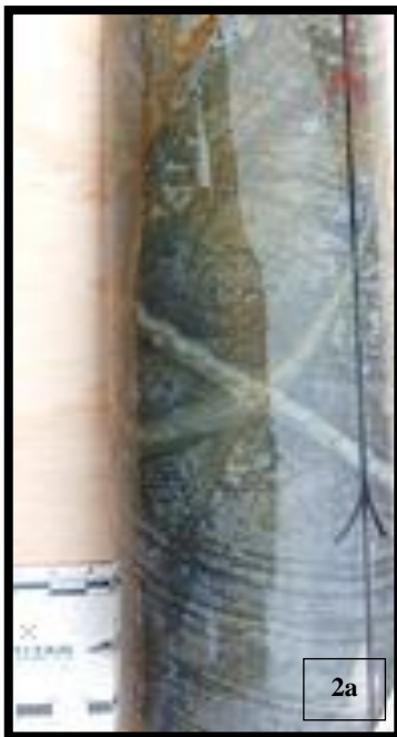
Plate 1: HTD001 core (31.64m to 35m interval), intersecting andesitic volcanic with partially oxidised quartz-pyrite stockworks and narrow quartz-pyrite-chalcopyrite veinlets
