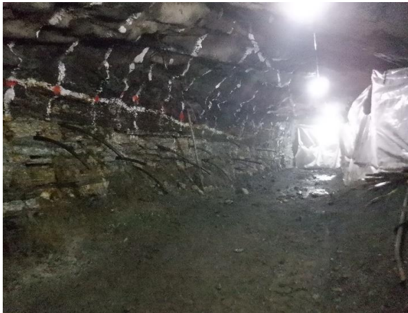
Figure 2 – Long holes drilled during the trial mining
