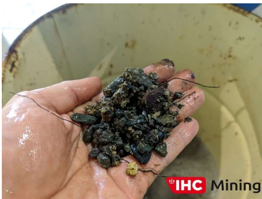
Plate 3 – Pebbles and organic matter from Trommel
