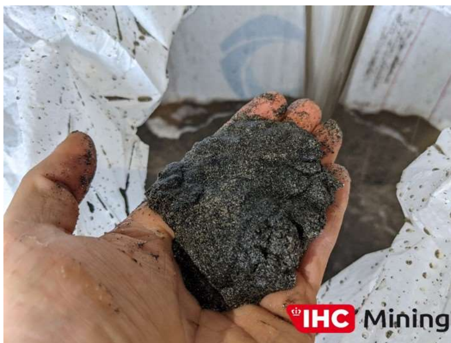
Plate 5 – Washed sand ready for industrial sand and magnetite-heavy mineral recovery ( +2\text{mm} -45\mu\text{m} )
