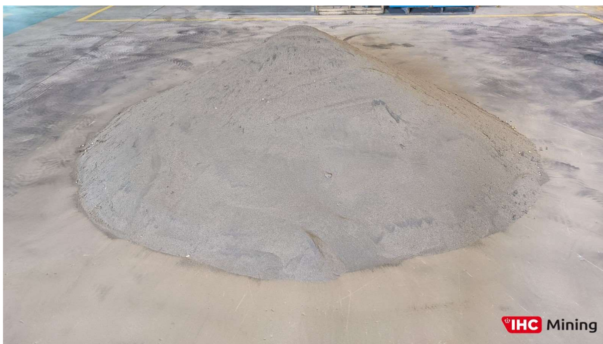
Plate 1 – “Run of mine” bulk sample prepared for pilot plant processing
