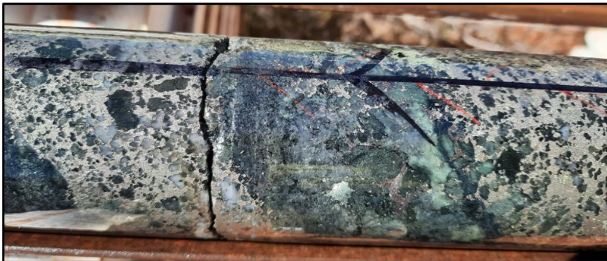
Figure 2 - Matrix sulphide mineralisation at 399m downhole in DBDD001 (field of view approximately 20cm across)
