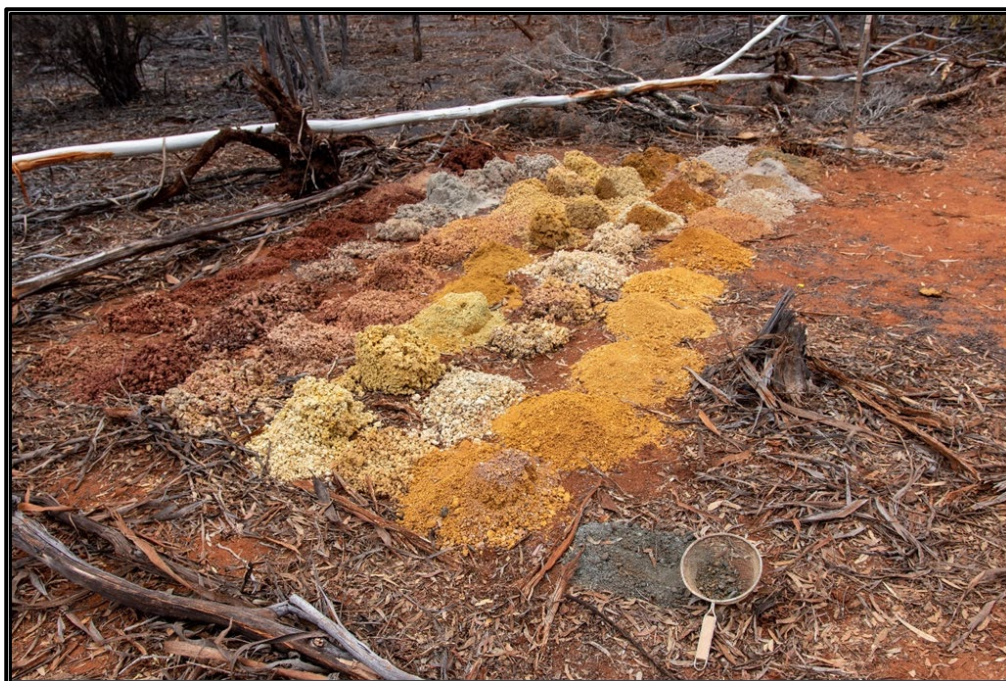
Figure 8 —Aircore Drill Samples with 1 Metre of Sulphide at End of Hole (right foreground with sieve)
