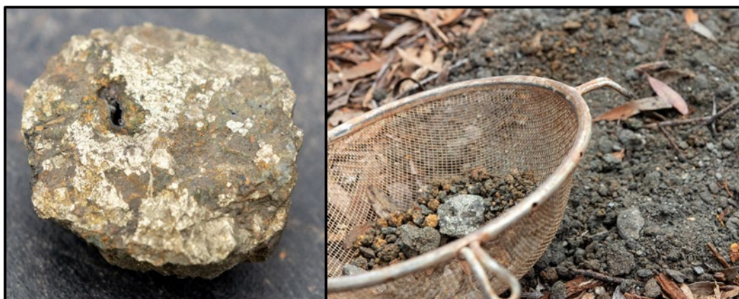
Figure 7 – Massive Sulphide Chip (25mm across) from 60m in NAC105. Bottom of Hole Sample Pile on Right. Drillhole was Unable to Breakthrough Sulphide
