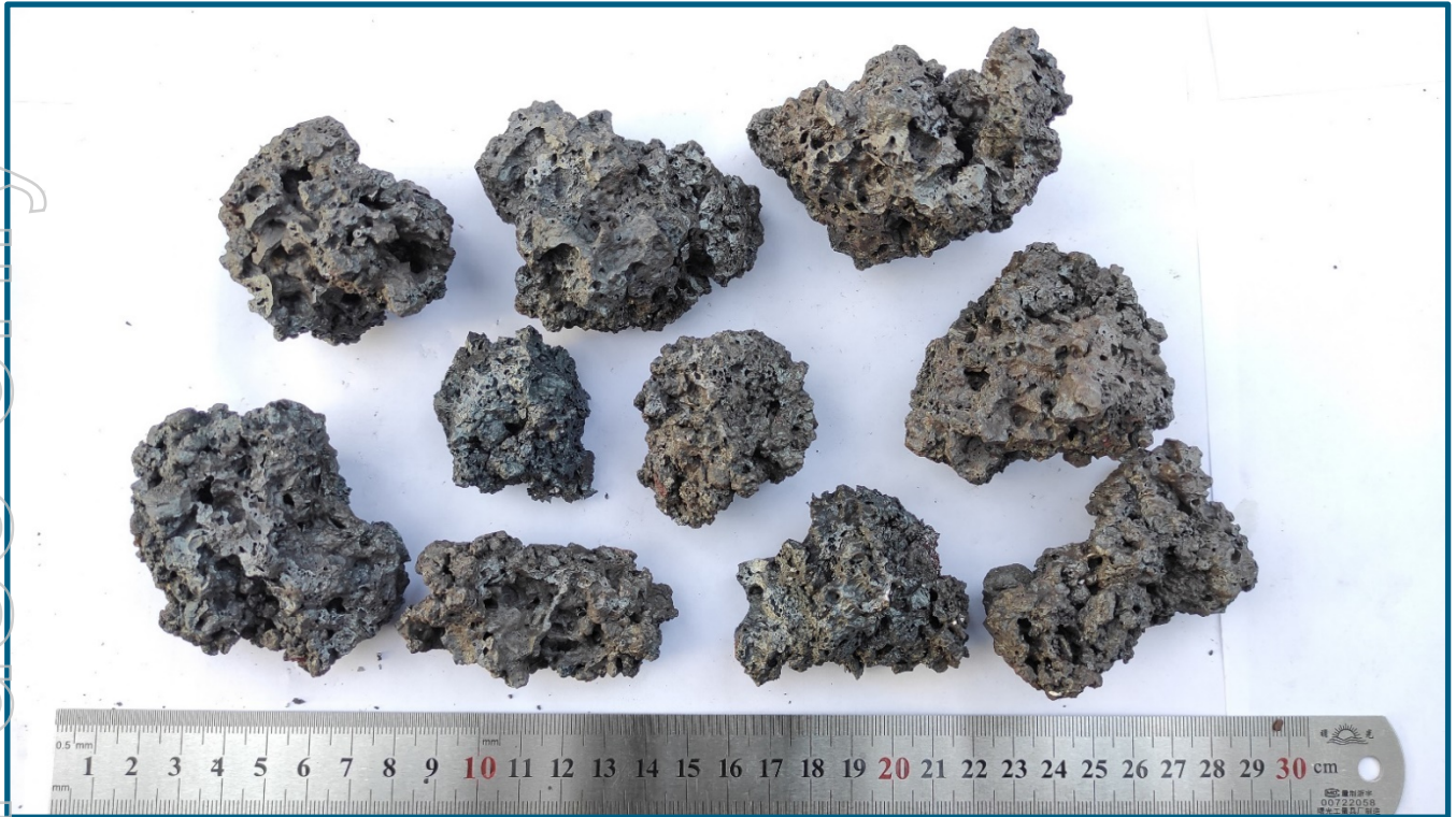
Figure 2: Sinter from pilot sinter pot tests containing 20% Baniaka Fines iron ore
