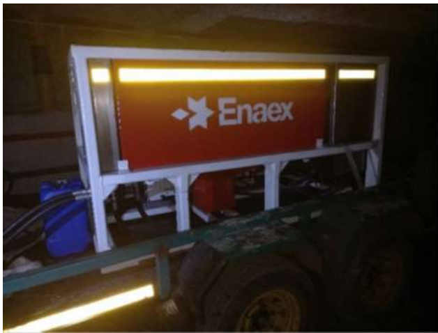
Figure 6 & 7- Bulk emulsion explosives charging unit
