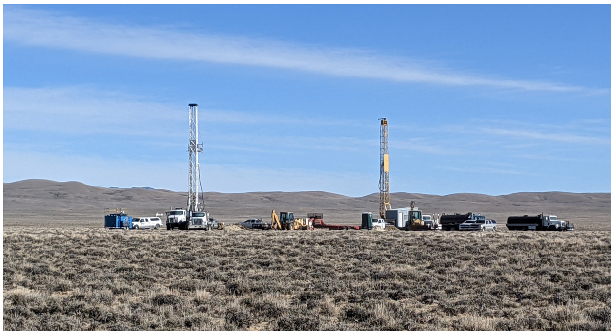
Figure 2. Mud Rotary Drill Rigs (x2), Ancillary Equipment and Support Vehicles at the Thor Project.
