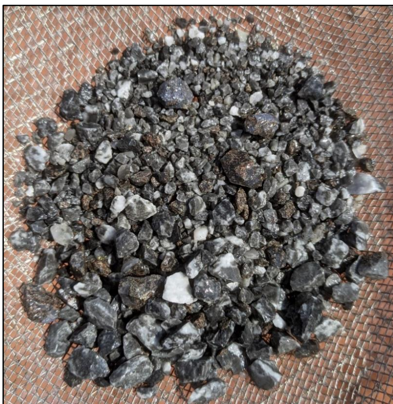
Figure 10: IQRC001 (137 to 138 metres). Sphalerite (red-brown-yellow) and galena (light grey) with associated carbonate veining within the Iroquois dolomite unit (dark grey). 12.7% Pb and 8.9% Zn
