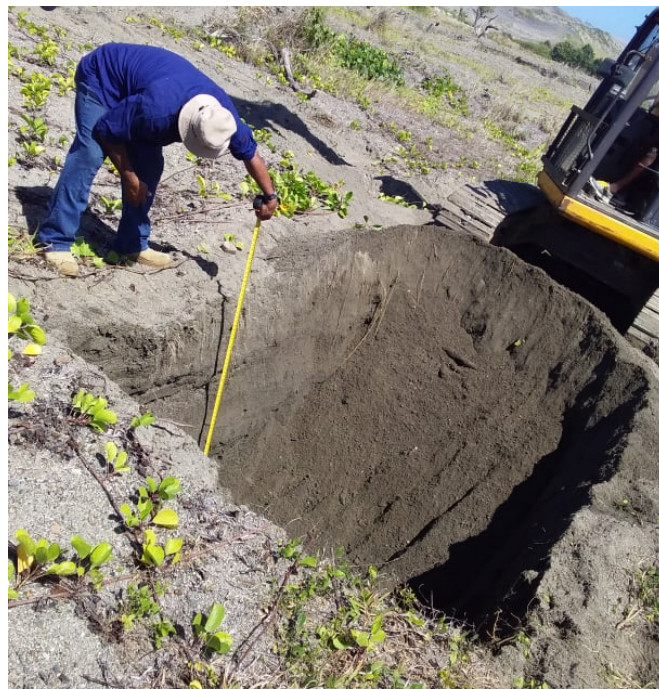
Plate 2 – Depth measurement prior to sample collection
