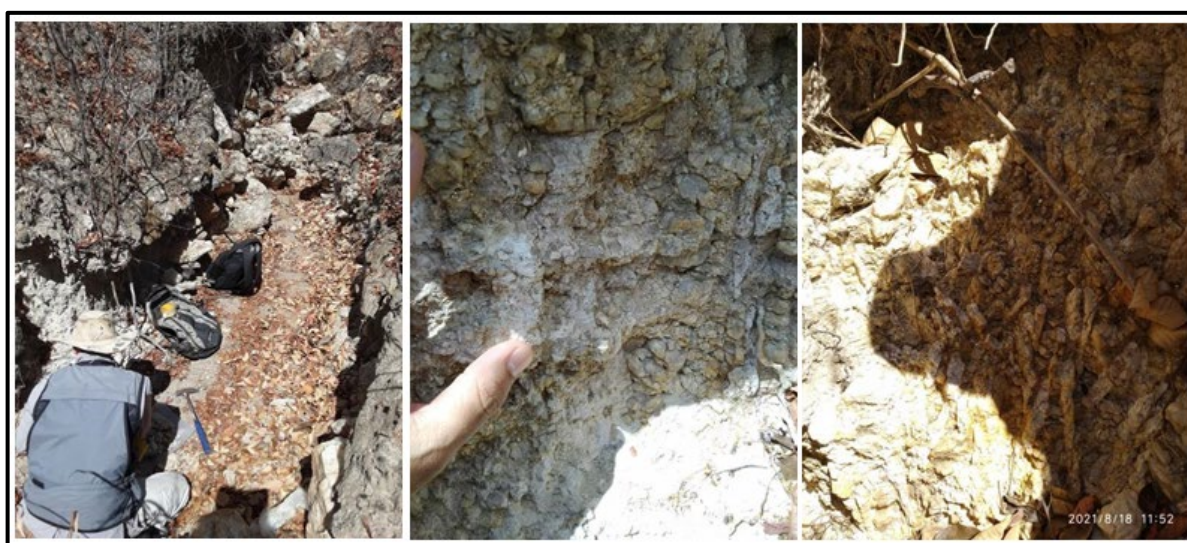
Figure 3: LRS geology team on site at the Bananal Valley Project - Mineralised pegmatite identified in mapping, with very weathered spodumene
