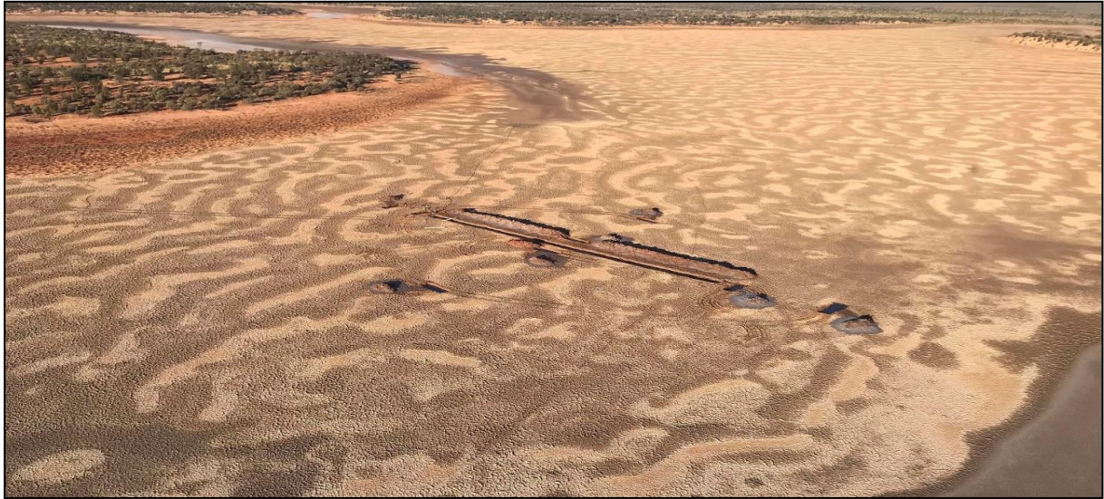
Figure 5: Trial Trench one with surrounding monitoring pits
