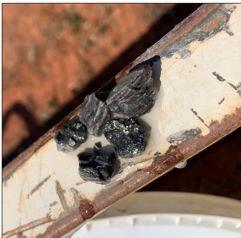
Figure 2 - Santy Project, sulphides with quartz veining within altered felsic schist.
